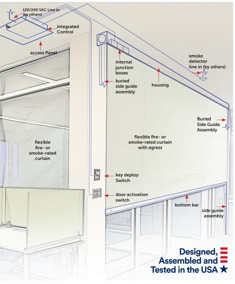
**Fail Safe Features.** The **M2500 Egress** is a gravity fail safe system. The **M2500 Egress** also features a fault report to indicate that the system requires a corrective action. This control also monitors the state of curtain deployment. An optional bottom bar sensing edge may be mounted to the curtain to guard against obstructions during deployment.
